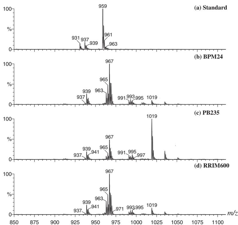
**Fig. 8.** ESI-MS mass spectra of DGDG from the fresh latex of three *H. brasiliensis* clones (b–d) compared to a standard from plant leaves (a). Details on assigned structures for ions detected in latex glycolipids are given in Table 4. The ions at  $m/z$  931 and 959 detected in the standard correspond to the structure of  $[C16:3/18:3\text{-DGDG} + \text{Na}]^+$  and  $[C18:3/18:3\text{-DGDG} + \text{Na}]^+$ , respectively.
