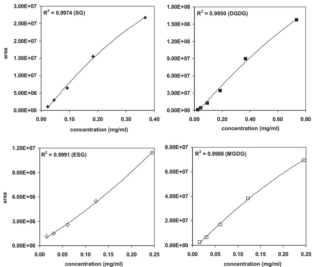
**Fig. 9.** Example of calibration curves of standard glycolipids for quantitation by HPLC/MS. A new calibration was realized for each series of samples. ■: DGDG, □: MGDG, ◆: SG and ◇: ESG.
