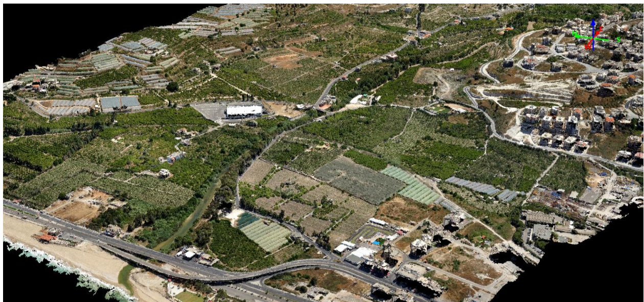
Figure 4.15 Screenshot for the developed point cloud for the Awali basin study site based on several UAV drone surveys, showing the low main part of the river and its outlet on the Mediterranean Sea.
