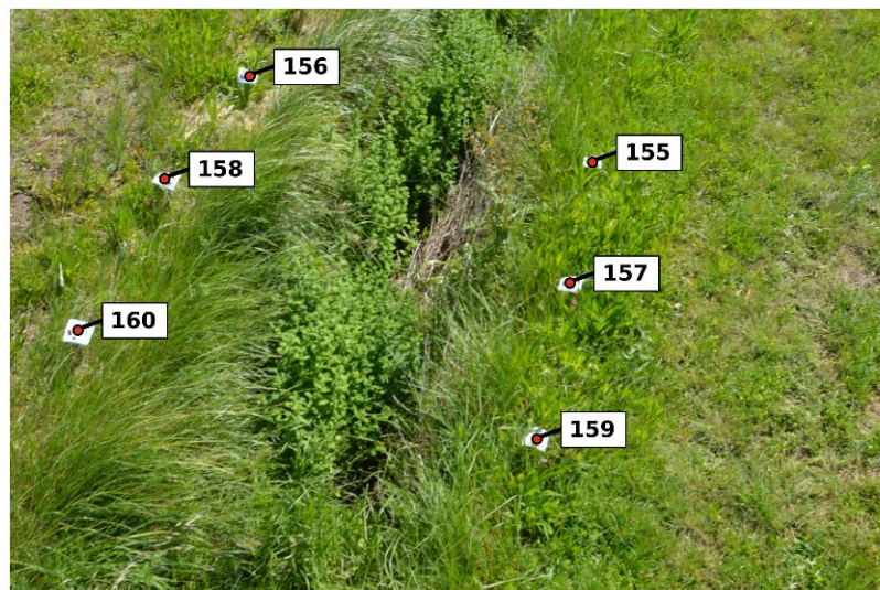
FIGURE A.3 – Illustration of automatic recognition of the targets on a picture using Photoscan Pro ® . (a) original image ; (b) image with recognized targets (boxes linked to a red dot).
